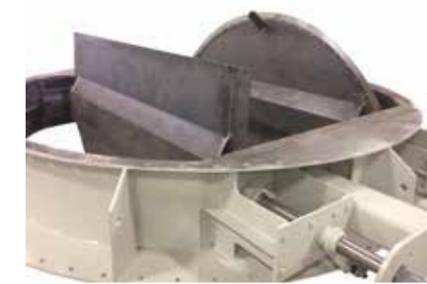
Clyde Bergemann Power Group America's (CBAM) Air-Gas Handling Product Division designed and supplied isolation dampers at each end of flue gas ducting, as well as non-metallic expansion joints installed along the duct that runs between the power plant and the heating systems of the tomato nursery. The duct conveys up to 20 % of the exhaust gas from the heat recovery steam generator (HRSG) stack to the greenhouse through an elevated duct approximately 183 meters (600 ft) long.
